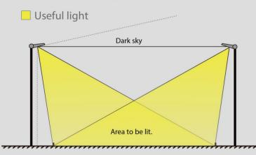
Venus Series LED Floodlight is specially designed for sports fields, minimizing loss of light and light pollution.
